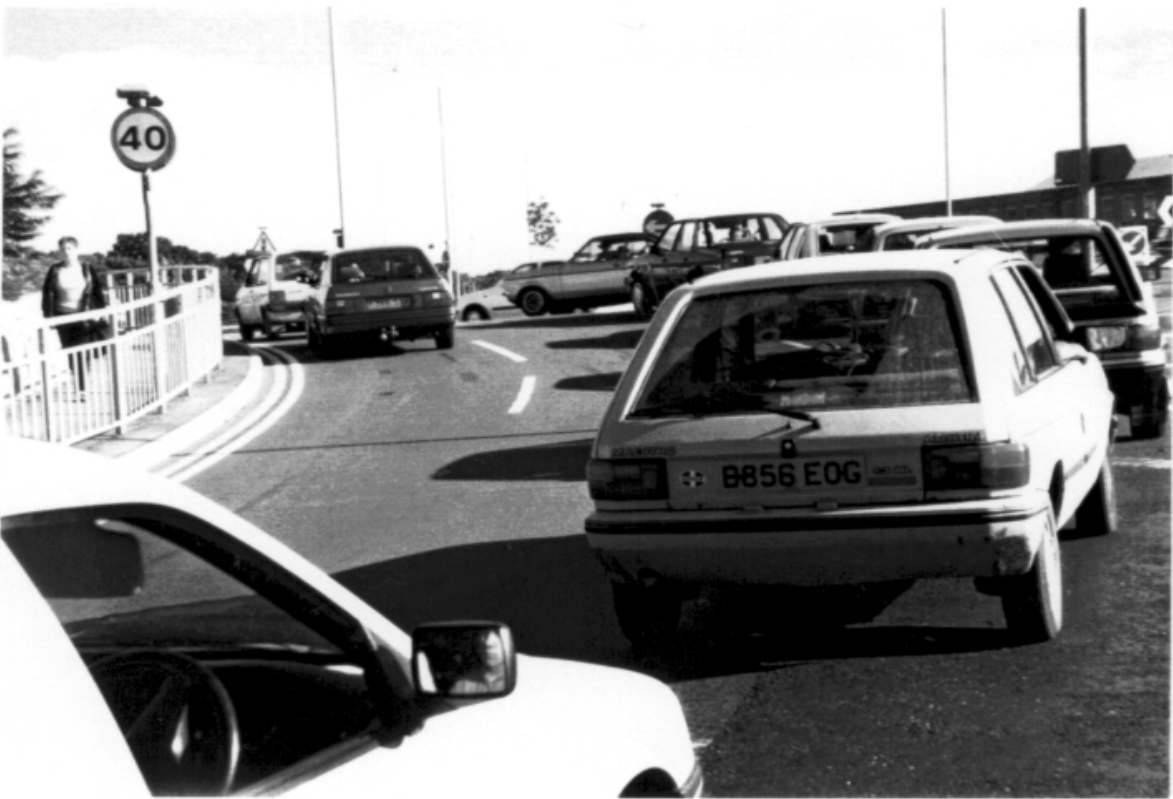
Photograph 1.2. This two-lane approach flares into three lanes at the entry no doubt giving better ARCADY capacity predictions. But traffic is not easily, comfortably or even safely able to use the middle section and doesn't!
