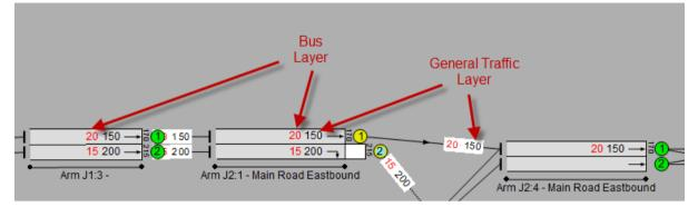
Each of the above entry methods support Lane Based Flow Layers.
