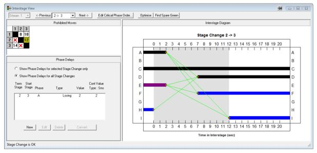
The Interstage & Phase Delays View show Interstages and Phase Delays for a single Controller at once, in a similar manner to other Controller related Views, and is used the same way regardless of whether Multiple Stage Streams are being used for the Controller being viewed. For more information on using Multiple Stage Streams see the Phase View section.
