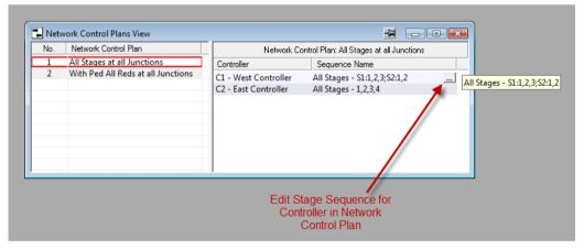
• Select a Stage Sequence from the drop down list. This is the Stage Sequence which LinSig will run for this Controller when this Network Control Plan is used in a Scenario.
