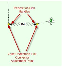
Pedestrian Links together with Pedestrian Link Connectors form a Pedestrian Network for each LinSig Junction. Pedestrian movements between junctions are not modelled. Due to
