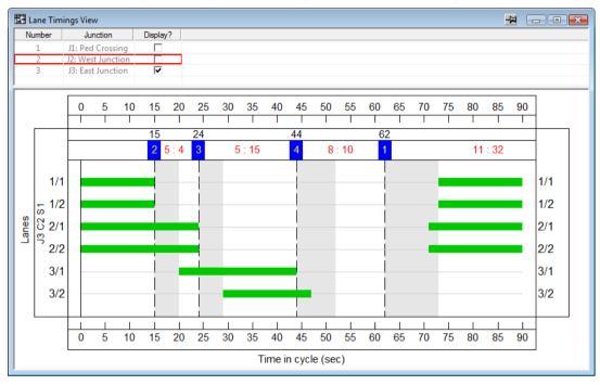
Its principal purpose is to allow the effective green times of individual Lanes to be adjusted using Bonus Greens to allow for effects such as underutilised green time and demand dependency.
