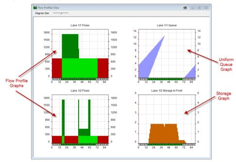
Graphs can only be viewed if traffic model results are available. If any errors exist preventing the traffic model from calculating results the Graphs will display an error message.
