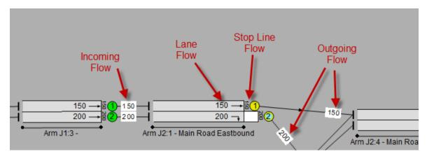
Where Flows are displayed by Layer each Layer Flow is shown in the colour of the Layer it is on. Layer colours are defined using the Edit Layers dialog box which is opened by choosing 'Edit Lane Based Flow Layers' from the Traffic Flows menu.
