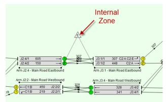
• Enter Zone origin and destination totals in the Matrix Estimation View. These should be estimated from the counted loss or gain of traffic between Junctions. This step is very important as if not carried out the matrix estimation process will tend to terminate or start and excessive number of OD movements in the Zone.
