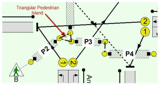
The diagram above shows three Pedestrian Link Connectors joining three Pedestrian Links to define which pedestrian movements can be carried out on the island.
