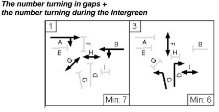
If the method of control is modified to provide an early cut off Stage (indicative arrow) as shown below, then right turners can turn in gaps during Stage 1, at full saturation flow during Stage 2 and will also receive a bonus for the number of vehicles stored in front of the stop line prior to Stage 2 starting.
