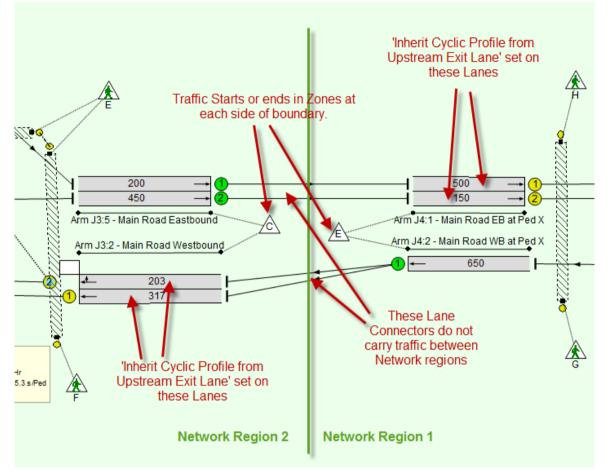
The use of the this method maintains cyclic flow profiles and coordination across the Network region boundary but greatly limits the number of Routes in the model by only modelling Routes within each Network Region and not modelling Routes between each Network region. The lack of Routes crossing the region boundary means that cyclic flow profiles of traffic crossing the region boundary would be lost if the above setting was not used.
