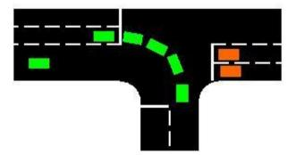
The Capacity during the time when the right turn is unopposed, possibly whilst an Indicative Green Arrow is running, is calculated using the value of 'Saturation Flow when Unopposed' defined for the give way Lane. This may be lower than the Lane's Saturation flow if the right turners share the Lane with Ahead traffic as the Lane's Saturation Flow relates to the Ahead movement.
