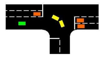
Vehicles waiting in the junction at the end of the main road stage can turn right during the Intergreen. The Intergreen clearance depends upon the geometric nature of the junction. In the example above it is assumed that the two yellow vehicles stored in front of the stop line will clear during the Intergreen period. Any other vehicles waiting behind the stop line will wait for the next cycle.
