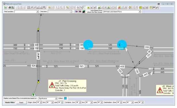
Flow Consistency errors are highlighted at the upstream and downstream end of each Lane. Where a consistency error occurs LinSig displays a coloured circle the size of which depends on the size of the consistency error.
