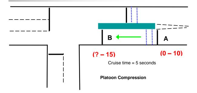
Hence, if the traffic at A is set to run green from 0 to 10 seconds with the usual start and end displacements of 2 and 3 seconds respectively, then the signals at B will need to be set at 7 to 15 with zero start displacement and 3 seconds end displacement. The effective green at both stop lines will be 11 seconds, giving the same degree of saturation.
