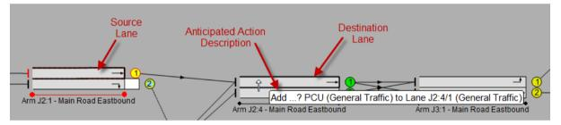
• Release the mouse button while pointing at the Destination Lane. LinSig will display the 'Specify Lane Based Flow Details' dialog box which allows detailed settings for the Lane Flow being entered to be specified.
