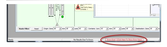
When Errors or Warnings exist in the Error View LinSig will highlight this by displaying a red or amber Error Indicator in the Status Bar at the bottom of the Main Window. The Error View can be opened by double clicking the Error Indicator.
