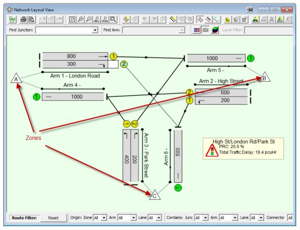
A Zone should be created for every point traffic enters or exits a Matrix Based Network or Matrix Based regions of a Network. Zones are not required for Lane Based Flow Network regions unless journey times are being calculated on Routes through the region. Further information is given on structuring a Network using Matrix Based and Lane Based Flow regions in the Essential Background section.
