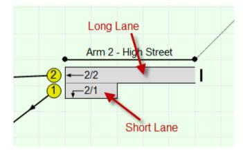
Where signalled Short Lanes are relatively long and are unlikely to empty during a typical green period they can generally be modelled as a Long Lane which can sometimes be useful in simplifying complex Lane arrangements.
