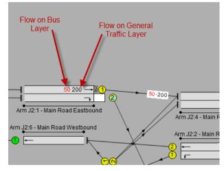
• Each Lane displays each Layers Total Flow. The Total Stop Line Flow across all Layers is displayed in front of the Lane.
