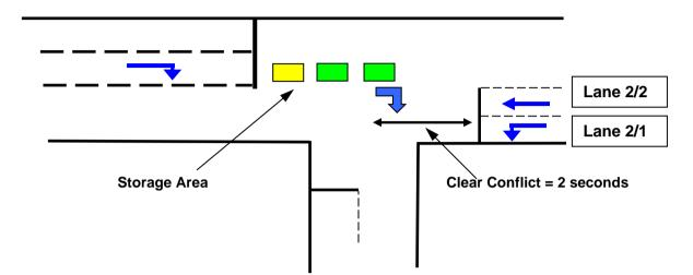
The mechanism of what happens with respect to the right turning traffic is directly dependant on the method of control. However, the parameters entered into LinSig are the same and LinSig uses them as appropriate depending on the method of control used.
