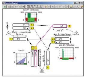
allows signal sequences to be built up using phases rather than stages possibly achieving a more efficient signal sequence.
