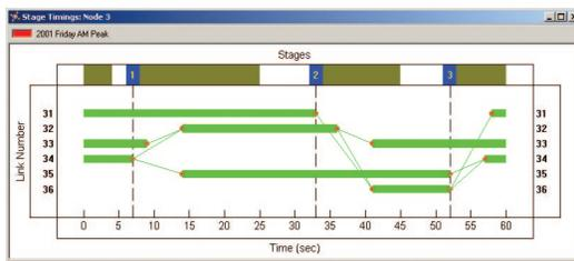
Figure 4: Stage Timings View showing when links run and how intergreens and link delays influence this.
