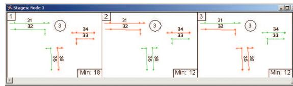
Figure 6: Stage View showing which links run in which stages
