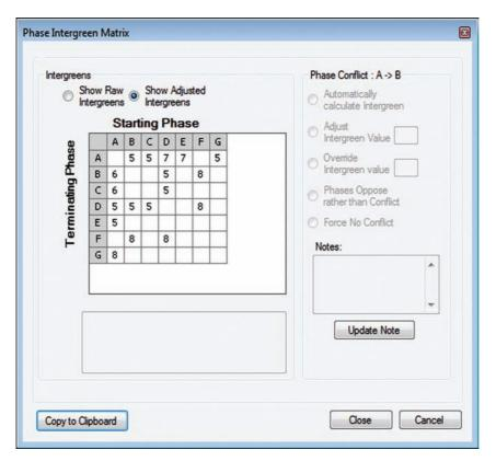
An intergreen matrix is produced which can be copied to any signal design software. larger the X distance the larger the required intergreen. TAL 1/06: Part 4 provides a look up table which allows different X distances to be translated into different intergreen values. The minimum intergreen between two normal three aspect phases will normally be 5 seconds although lower values may sometimes be used with indicative green arrow phases.
