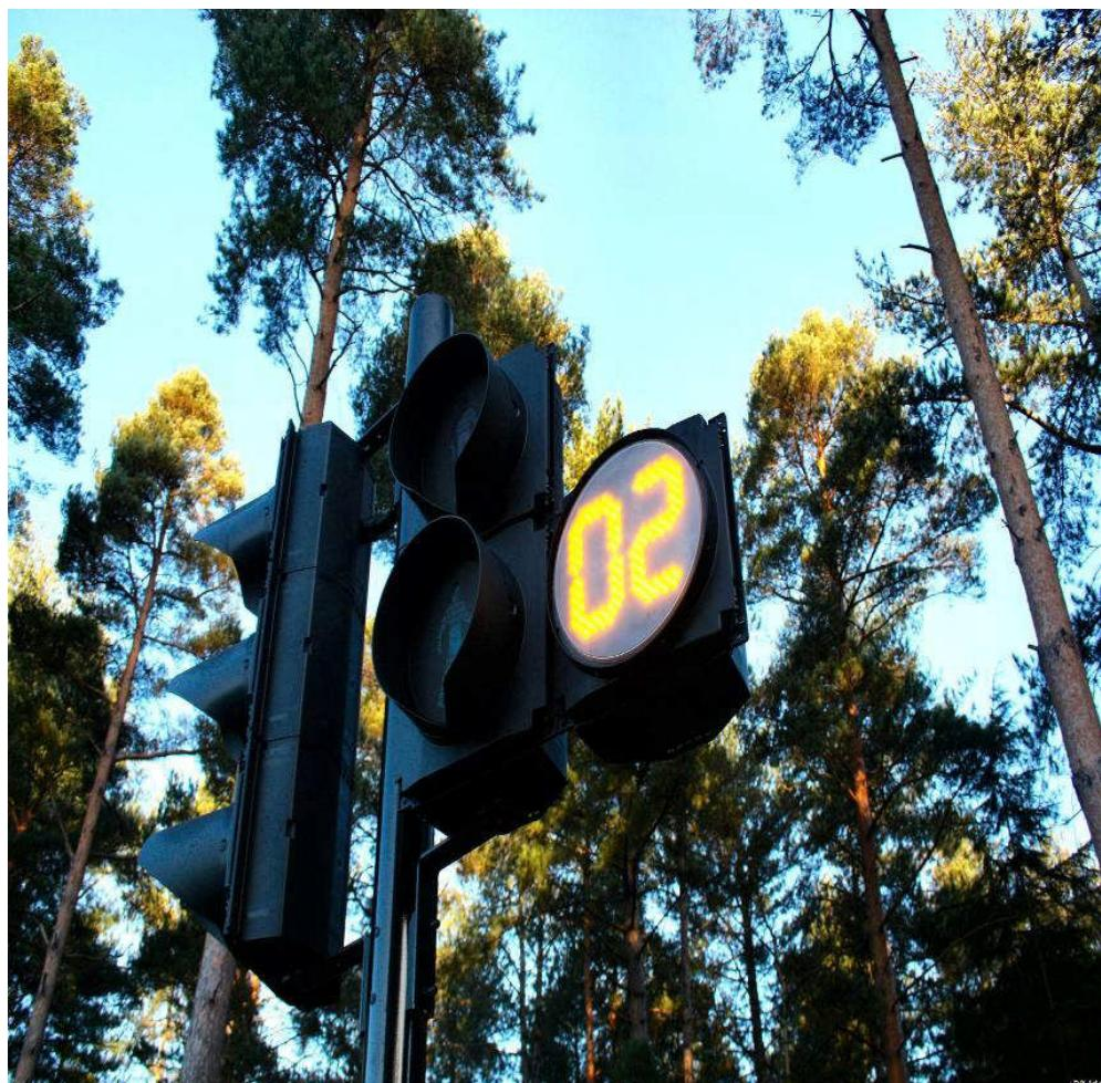
PCaTS unit at TRL's test track
