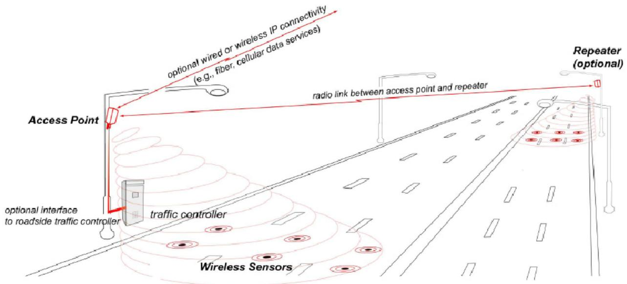
The Access Points are usually mounted on top of a suitably positioned signal head. The Repeater Units, where needed, are battery powered, with either two or seven year replaceable battery options available. Each repeater can support up to 10 sensors, also within a 30m range, relaying the detection data back to Access Point and extends the range of an Access Point by up to 300m.
