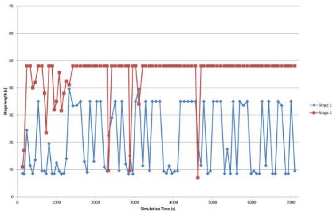
Figure 3: Existing MOVA operation - green time per stage
