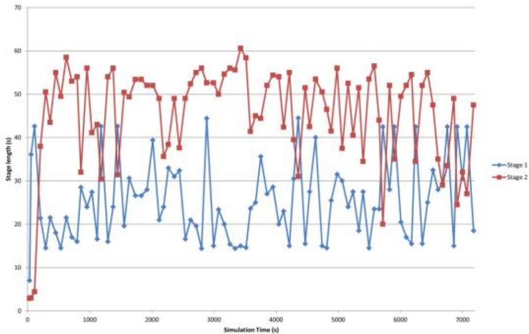
Figure 4: Proposed MOVA operation - green time per stage
