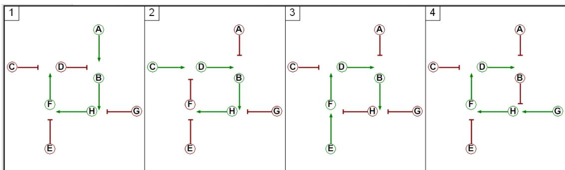
Fig. 1 – ACS Stage Sequence at a 4-arm roundabout.
