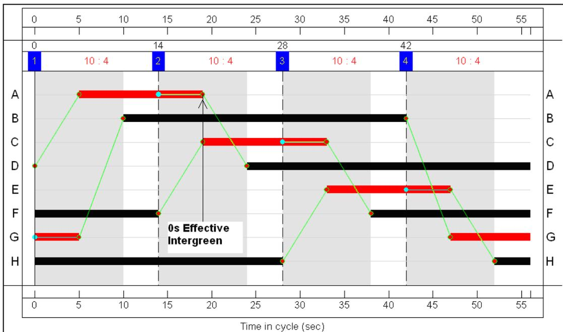
Fig. 2 – ACS Phase/Stage relationship for a 4-arm roundabout.
