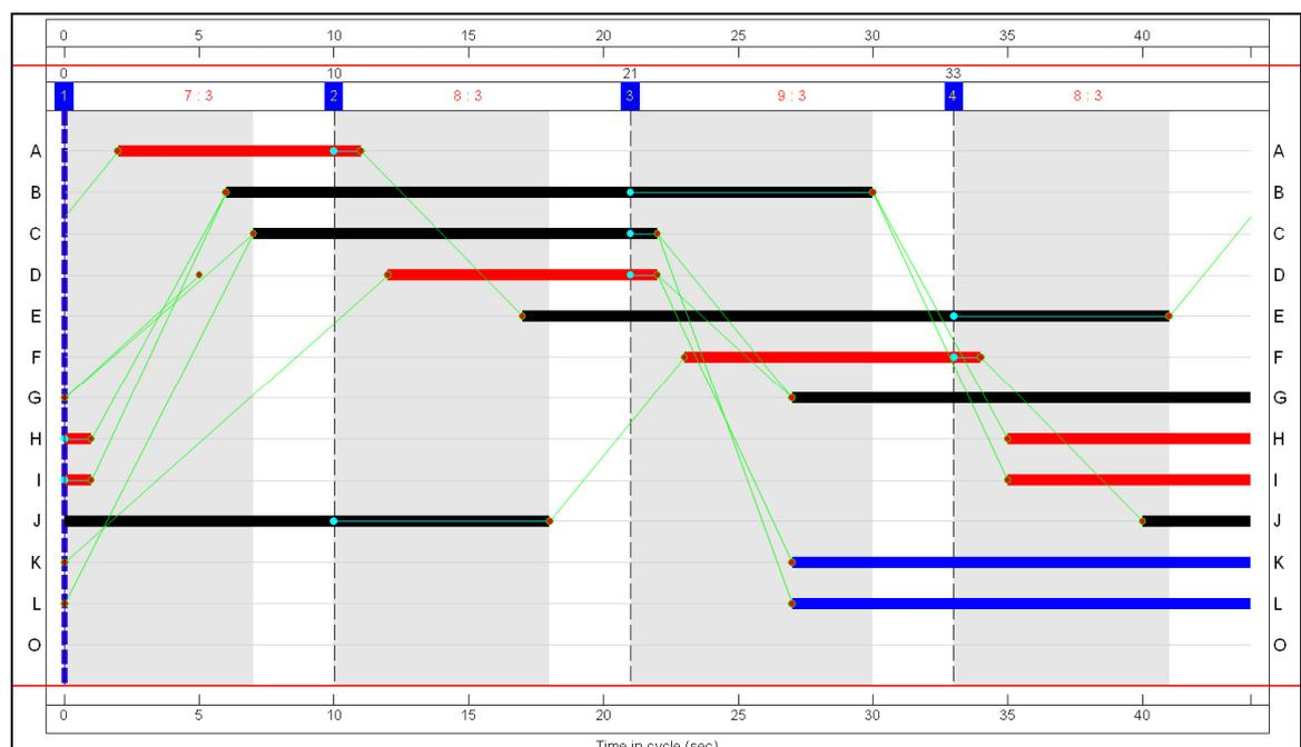
Fig. 6 – MOVA ACS stage / phase view – minimum sequence.
