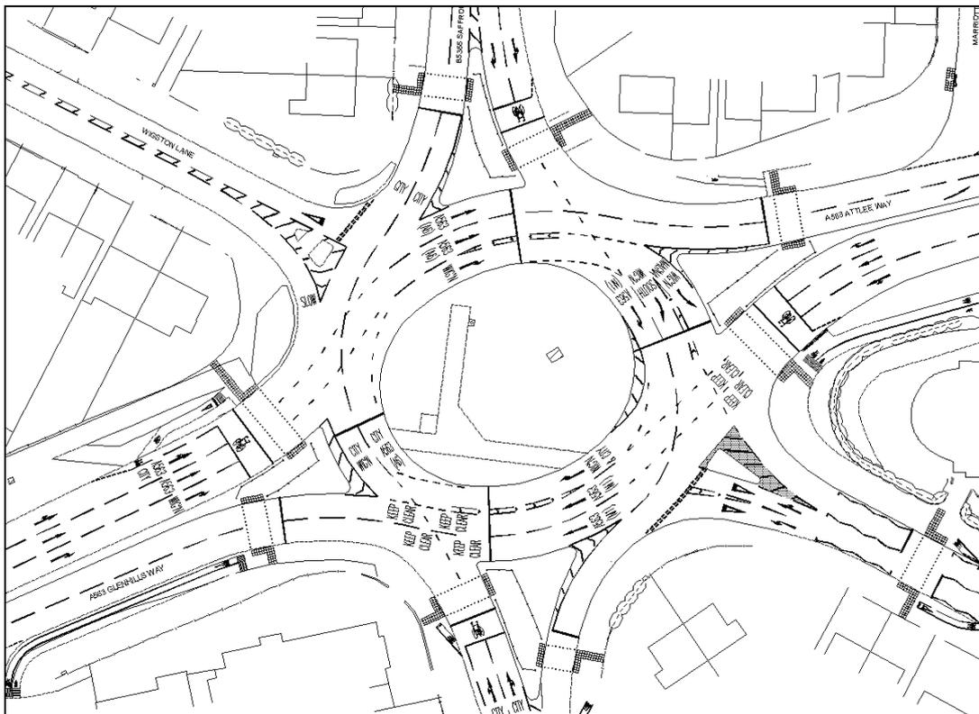
Fig. 3 – An Example of a SCOOT controlled single-stream 6 arm roundabout ('Pork Pie' roundabout designed by WYG for Leicester City Council, commissioned 2007).
