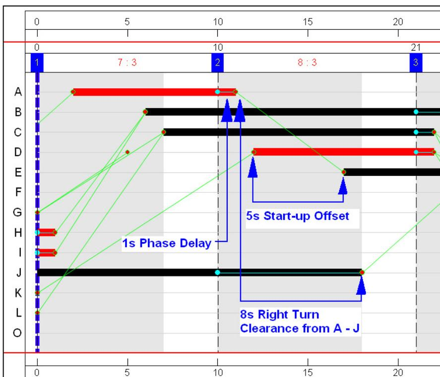
Fig. 7 – MOVA ACS Example – Stage 1-2 interstage structure.
