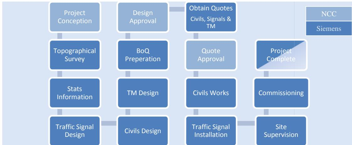
**Figure 1 - Project Scope of Works**
