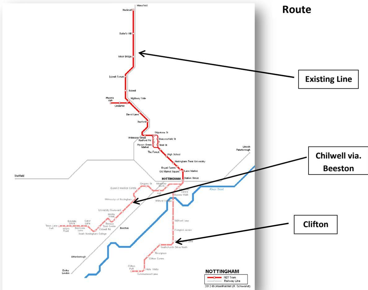
NET2 will continue south from the railway station and split into two routes, one to Clifton and one to Chilwell. The line to Clifton is 7.6km long and 63% of it is segregated. The line to Chilwell via. Beeston is 9.8km long and 59% of it is segregated. The two routes will pass through almost 40 sets of traffic signals. The overall process of planning and designing the tram route is a very lengthy process and
