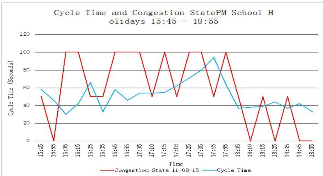
Figure 8 - Congestion State and sampled Cycle Time from West Controller during PM peak (linking is applied to the A64 Southbound entry node when red line is High or Medium) – Responsive Mode
