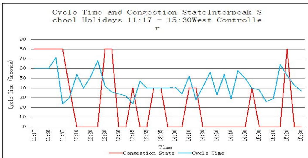
*Figure 10 - Congestion State and sampled Cycle Time from West Controller during Inter peak, linking is applied to the A64 Southbound entry node when red line is High or Medium – Responsive Mode*
