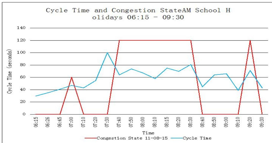
Figure 6 – Congestion State and sampled Cycle Time from East Controller during AM peak (linking is applied to the A64 Northbound entry node when red line is High or Medium) – Responsive Mode
