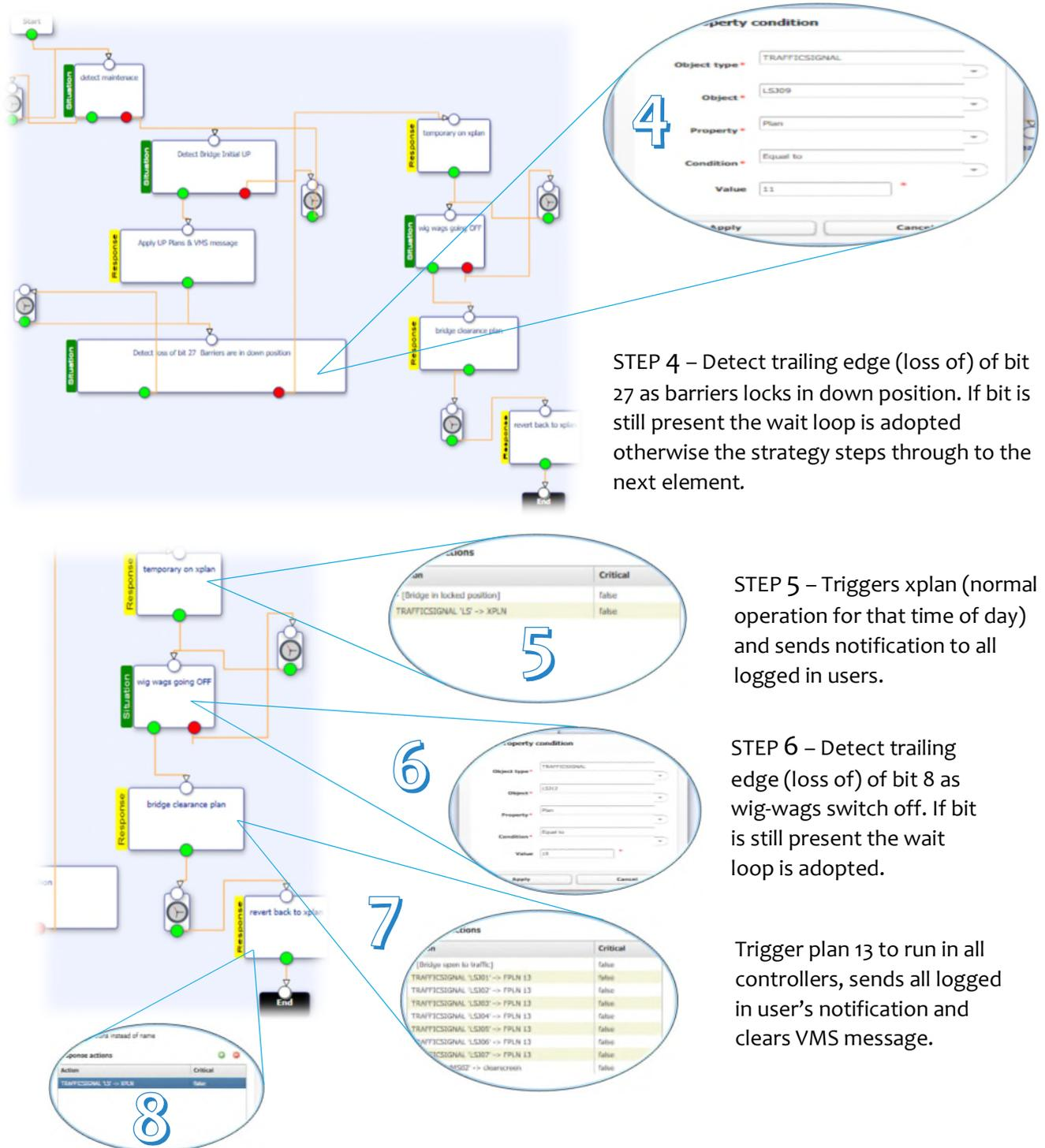
STEP 4 – Detect trailing edge (loss of) of bit 27 as barriers locks in down position. If bit is still present the wait loop is adopted otherwise the strategy steps through to the next element.
