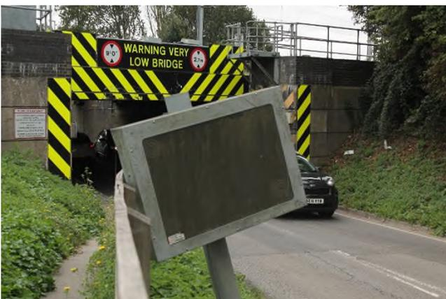
This may be due to the short distances from the OVD to the VMS, or from the signs to the bridge, which allow little reaction time.
