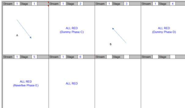
The site is configured with two real phases, A and B, and also two extendable ‘clearance’ phases, C and D. There is also an additional dummy phase for a revertive all red, E.
