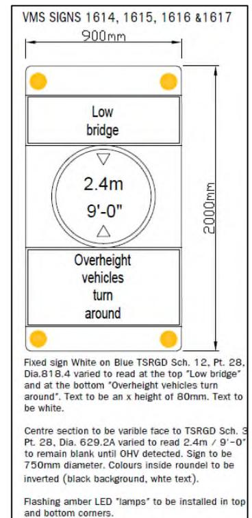
The detectors will now trigger approximately 5 seconds journey time away from the signs, giving drivers time to read and react to the sign. The crossing, OVD and signs will all be linked back to the shuttle working signals for monitoring.
