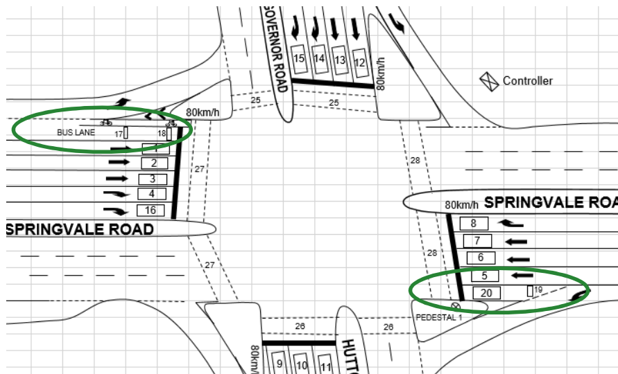
Fig 5: Bus detectors which demand bus early starts and exclusive bus phases
