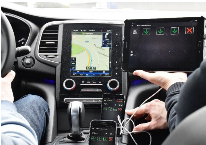
Figure 2: DynnIQ's GreenFlow in-vehicle app displaying traffic messages in real-time at the Belgium TestFest
