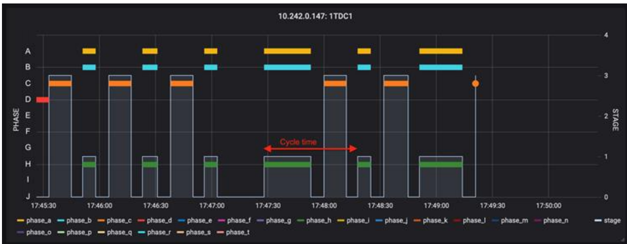
Figure 4 - Example of the live monitoring by the prototype Data Platform of signal phase, stage and cycles for each controller which is pushed to PTV Optima after each cycle and used in the live traffic forecast
